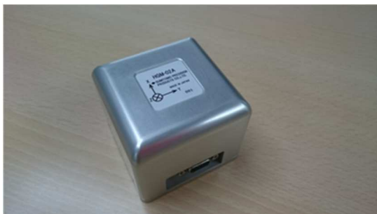
Fig. 2. Trial model of MEMS IMU (HGM-02A)
