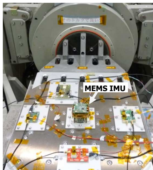
Fig. 3. Vibration test setup
