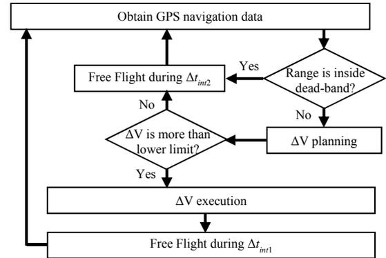
Fig. 2. Flow-Chart of stationkeeping algorithm
